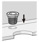
14. Install the tower-shape gasket into the tank hole.
