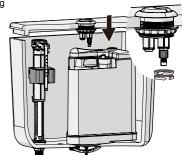
24. Position the ceramic tank cover onto the tank. Remarks:Loosen the nut, adjust the rod to the suitable length, screw up the botton nut tightly.
