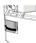
8. Turn the lock buckle to the locked position.
