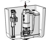
19. Position the valve body into the base and lock it in place by rotating it clockwise.
