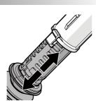
3. Pull adjustable pipe up and down until adjusting to the suitable height.
