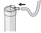
21. Attach the refill tube to the overflow pipe for refill.
