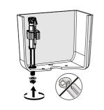
11. Install the fill valve into tank, rotate the gasket and nut.
